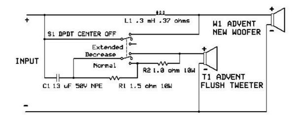
New Large Advent - these are original unmodified Serial Numbers: U3 96378 U3 96308 DESCRIPTION MEASURED #1 MEASURED #2 T1 NEW LG TWEETER 2.33 Rvc 2.33 Rvc W1 NEW LG WOOFER Note 3 4.47 Ruc C1 13uF 50Y NPE 13.01uF 13.05 uF .65 ESR @ 1kHz R1 1.5 Ohm 10W 1.53 R 1.56 R R2 1.0 Ohm 10W 1.02 R 1.02 R L1 .3 mH .37 ohms .298 mH .36R .305 mH .38R @ 1kHz S1 DPDT CENTER OFF SWITCH
